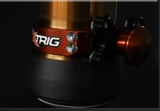
New billetproof CNCmachined, anodized axle brackets
