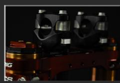
New designed PSF Top Cap with angular screws for easy clicker acces
